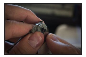
Carefully attach the contact over the old one. Pressing the thumb on the contact while sliding the knife away from under it worked for me. Maybe one or two times did the disc fly off, but other than that it went fine.
